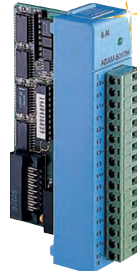
ADAM-5017H, 8-channel high speed analog input, $285, shown smaller than actual size.
