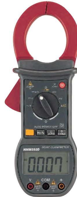
HHM592D Clamp-On Multimeter 2500 counts resolution Microprocessor-based DMM AC current up to 700 A DC current up to 700 A DCV accuracy up to 0.25% with EL panel LCD
